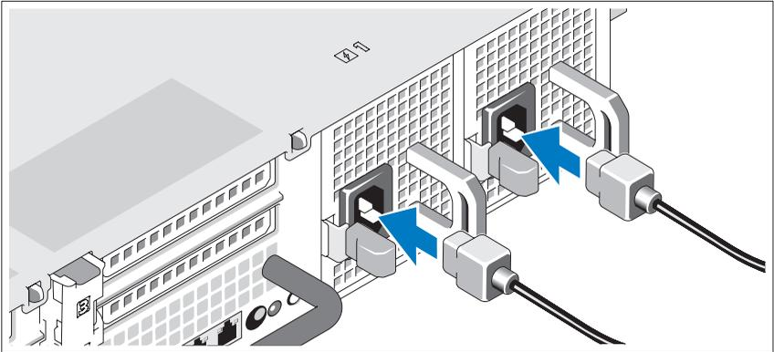
Connect the system's power cable(s) to the system.
