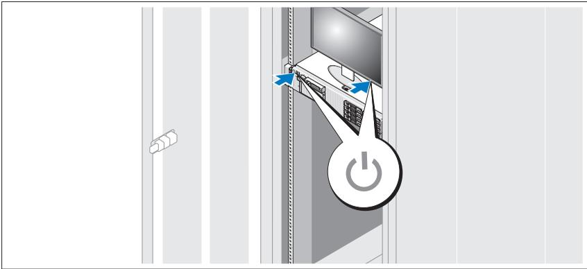
Press the power button on the system and the monitor. The power indicator should light.
